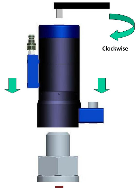
Continue rotating the Puller, increasing its engagement with the bolt until the bridge is flush with the washer. To ensure the tool is fully flush, it may be necessary to rotate the gearbox slightly whilst lowering to fully engage the gear driven socket with the nut.
