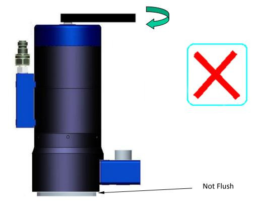
Once the Tensioner is in situ, it should still be possible to rotate the bridge to a suitable angle to access the bolt if required.
